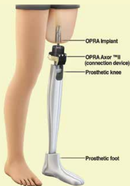
Figure 7. The OPRA Implant System is an example of an osseointegrated prosthetic leg that is attached directly to the bone by inserting a threaded titanium implant into the bone marrow at the amputated end of the residual limb.
